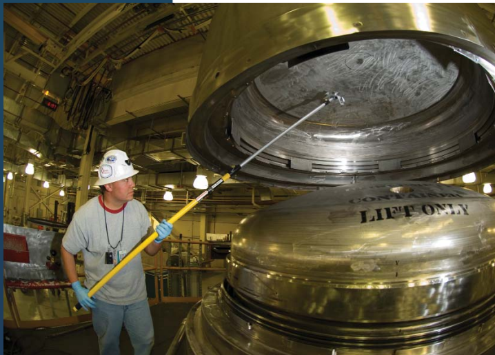
A WIPP radiological control tech takes a radiological "swipe" under the lid of the shipping container.
