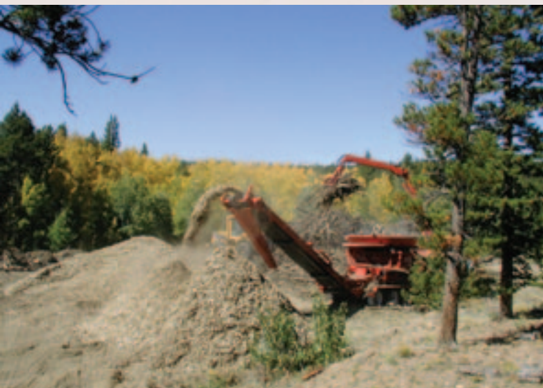
Converting forest slash into usable wood chips for energy.
