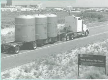
A truck carrying casks that will hold transuranic waste makes a test run to WIPP.
