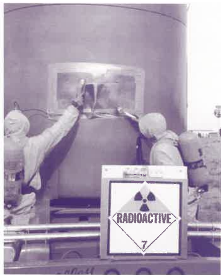
A cask for radioactive waste is inspected during a WIPP training exercise.
