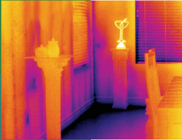
Thermal Infrared image of residential inspection energy audit. Note the cold air infiltrating (Black/blue areas)
